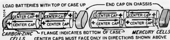
Later Production Battery Holder Showing Ordinary and Mercury Type Batteries in Correct Positions.
